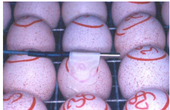
Figure 4. Positioning of data-logger probe on egg tray.
