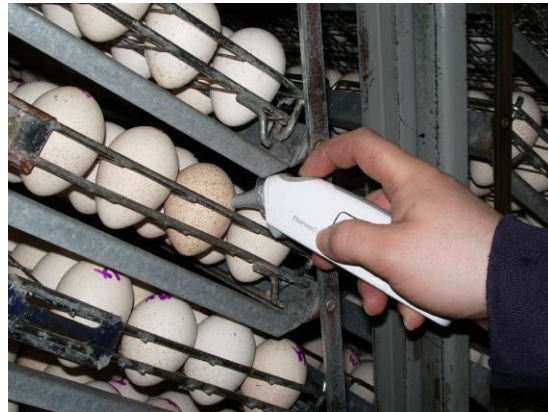
Figure 2. Measuring egg temperature using an infrared thermometer.
